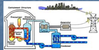
Pressurized Water Reactor
